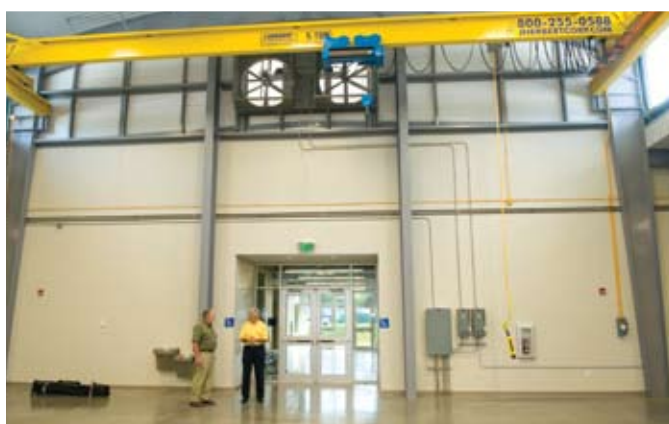
Sasser, with Wendell Collins of PPI, examines the 10,000-pound crane high over head at the newly opened Charles Perry Construction Institute on campus, used in the construction of disaster-replacement homes.
